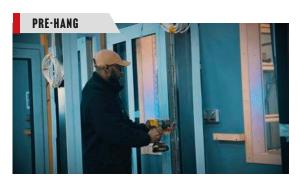
This is the final process on production line, where all ironmongery is placed and fixed onto the doors.
