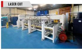
Our Trumpf laser cutting machines process stainlesssteel flat and tube profiles within only 0.1mm of tolerance.
