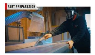
Part preparation: High quality timber is prepared for putting inside the frame of doors.
